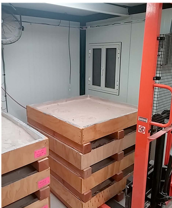
Figure 3. Stack of aluminum-lined sample holders inside sample conditioning chamber. Orange device is a hydraulic forklift used to maneuver sample holders within chamber. Temperature and relative humidity sensors were buried at the center and bottom of each sample holder box (not visible).
