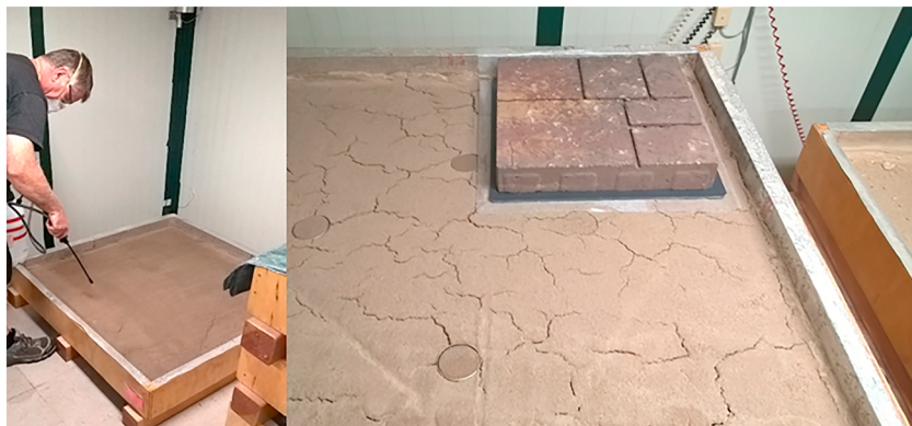
Figure 8. (left panel) Application of water prior to third testing period. (right panel) Masonry block atop wetted surface to simulate light compression.
