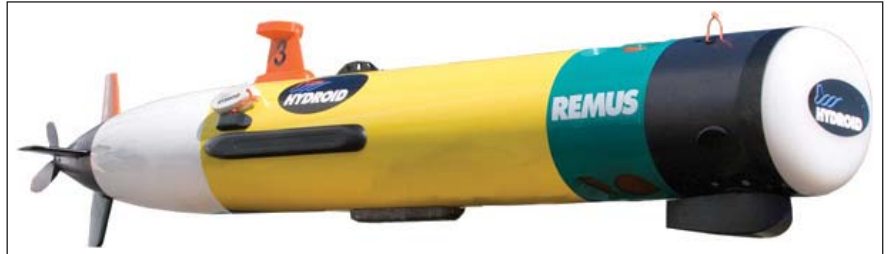
Figure 3.1. Autonomous underwater vehicle (AUV). Credit: Kongsberg Maritime.
