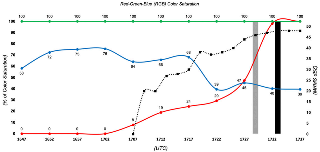
FIG. 7. St. Augustine storm time series of GOES-16 Day Cloud Phase Distinction RGB composite red component color saturation (%; red solid trace), green component color saturation (%; green solid trace), and blue component color saturation (%; blue solid trace), MRMS -10^{\circ}\text{C} isothermal reflectivity (dBZ; black dotted trace), initial ENT L in-cloud lightning (vertical gray bar), and initial ENT L cloud-to-ground lightning (vertical black bar) between 1647 and 1737 UTC 21 Jun 2018.
