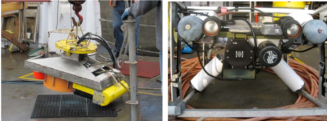
Figure 20. Simrad 38/120 kHz system deployed alongside Reson 7125 prior to mounting on the hull of the NOAA ship Nancy Foster (left). Phantom 2 ROV with video camera and DIDSON high resolution sonar as deployed at dedicated fish survey sites (right).
