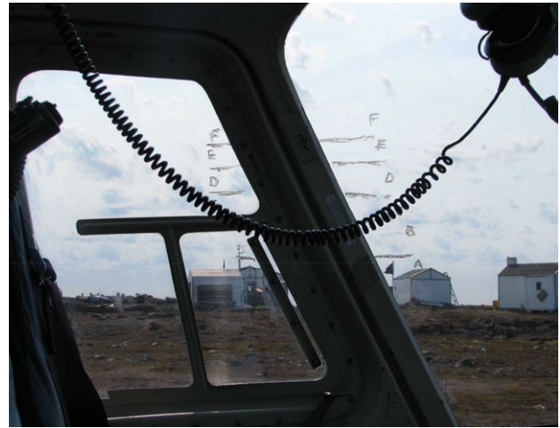
FIGURE 1 Example of distance classes marked nearest the left front seat of a Bell 206 Long Ranger helicopter
