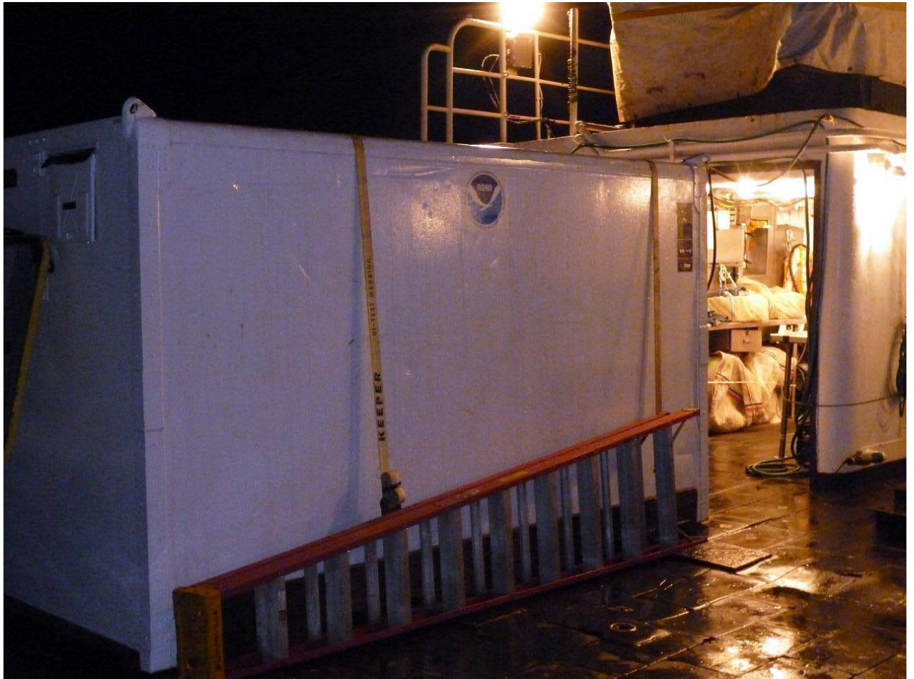
Figure 3. Container laboratory mounted on aft deck of the Delaware II.
