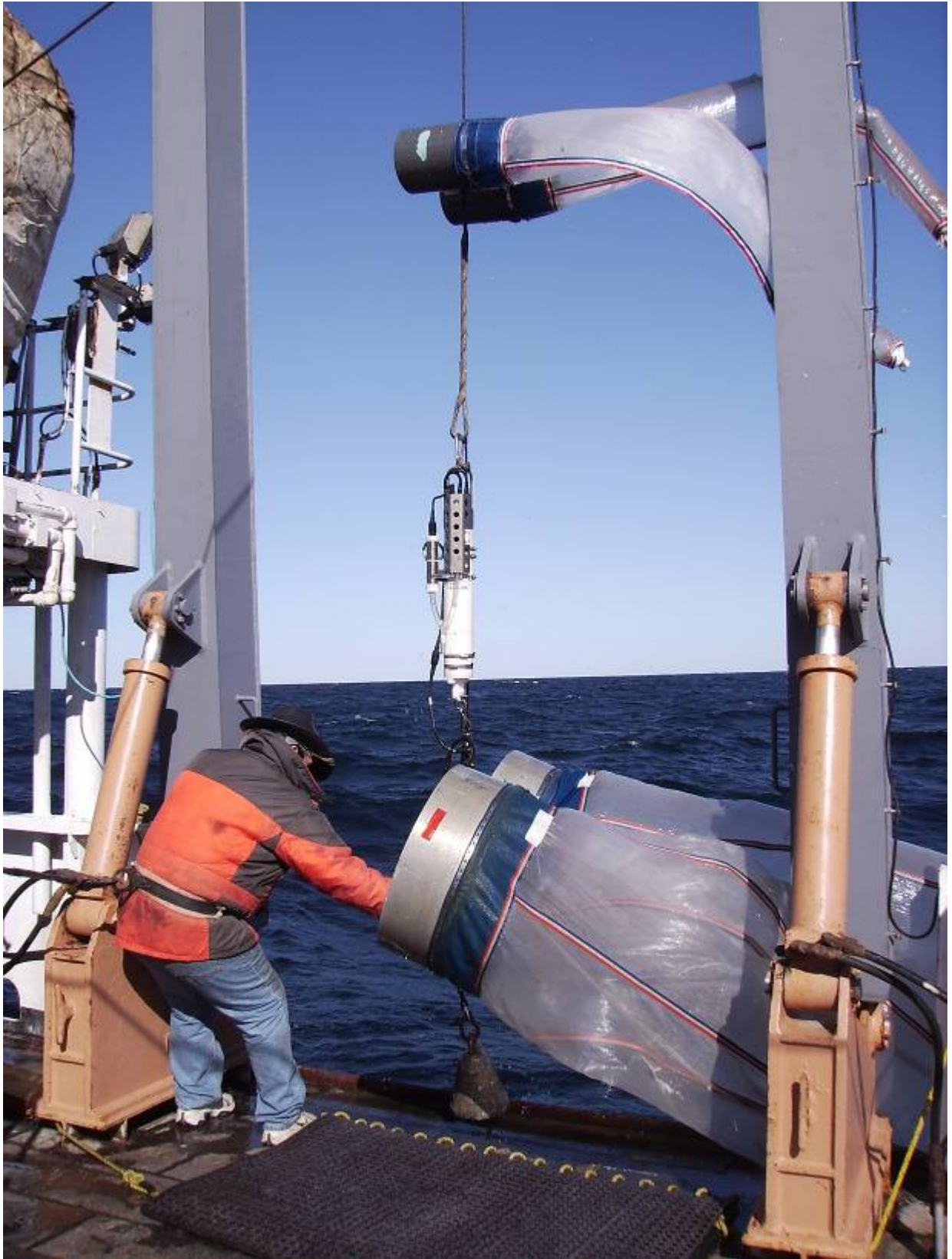
Figure 2. 20 cm + 61 cm bongo sampling array used for collecting CMarZ samples simultaneously with Ecosystem Monitoring samples.
