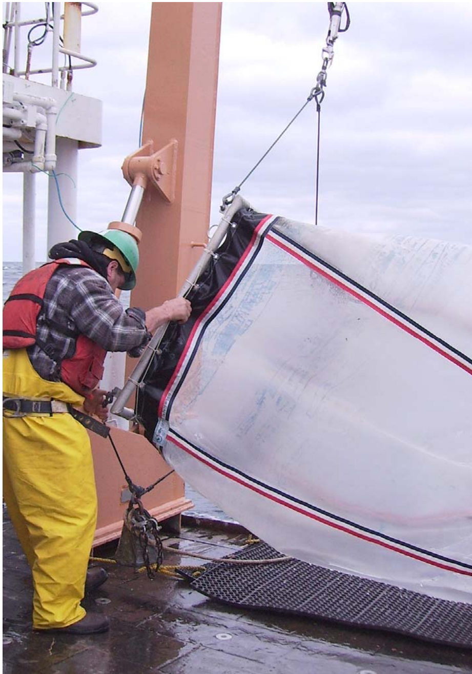
Figure 5. Meter net, properly rigged on DE0911 Fall EcoMon Cruise. Note that depressor is attached to lower part of frame and tow cable is attached to upper part of frame.
