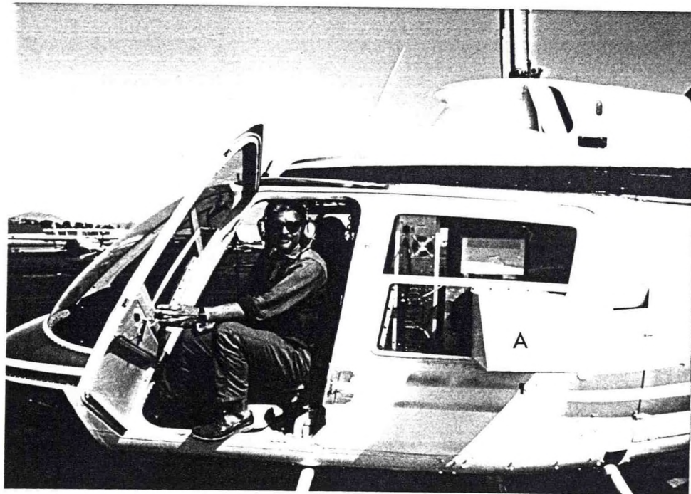
Figure 10. Installation completed, door and window installed. The beam directing mirror assembly (A) is the only external component.
