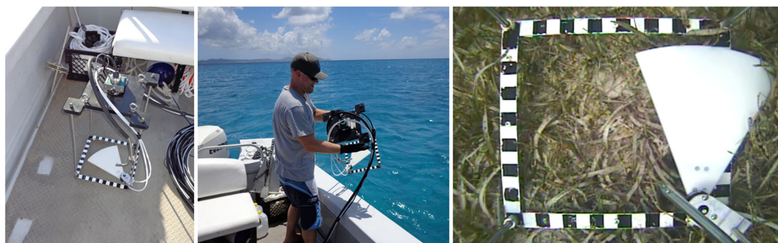
Fig. 2 Acquisition of underwater reflectance spectra, which served as reference data for assessing the lidar-derived seafloor relative reflectance mosaics. Left: camera frame and spectrometer probe on deck of boat. Middle: deploying camera frame over the side (note: fiber optic cable connects spectrometer probe to the instrument, which remains on vessel).
