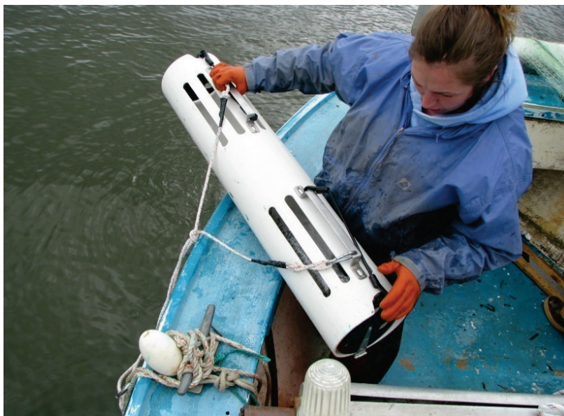
Figure 2. Custom fabricated PVC fish tube, which facilitated safe handling of adults and allowed study fish to be held individually in the river and within holding tanks.
