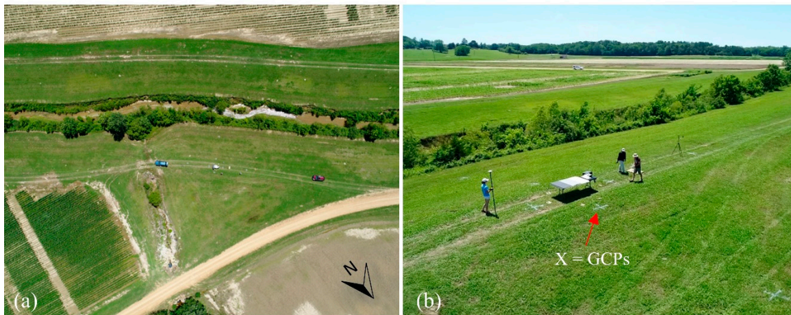
Figure 3. (a) R. R. Foil Plant Science Research Center (North Farm) study area on the campus of Mississippi State University. (b) View of the North Farm 2.0 research site configuration where Xs represent the eight ground control points (GCPs).
