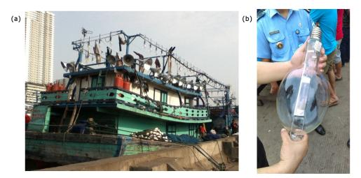
**Figure 11.** Photos taken during field survey in Indonesia. (**a**) Purse seiner at Muara Angke Port, Jakarta. Equipped with 60 bare 1500 watt metal halide bulbs, and 24 shielded bulbs pointing into the water. (**b**) Closeup look of a 1500 watt metal halide bulb.
