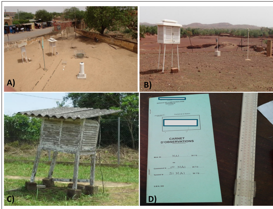
Photo 2: Status-quo of selected primary weather stations in West Africa and its basic components. A) A synoptic station overcome by urbanization in Burkina Faso. B) A climate station with defective and missing sensors in Burkina Faso. C) A tilted Stevenson screen hosting maximum, minimum, dry and wet bulb temperatures, and a pitch evaporimeter in Togo. D) The observer's logbook for recording data and a manual slide rule still in use to derive some additional variables in most of the observatories.
