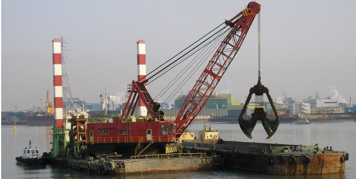
Figure 2. Large clamshell dredge on a spud barge. A second a barge for sediment collection and transport is moored alongside.
