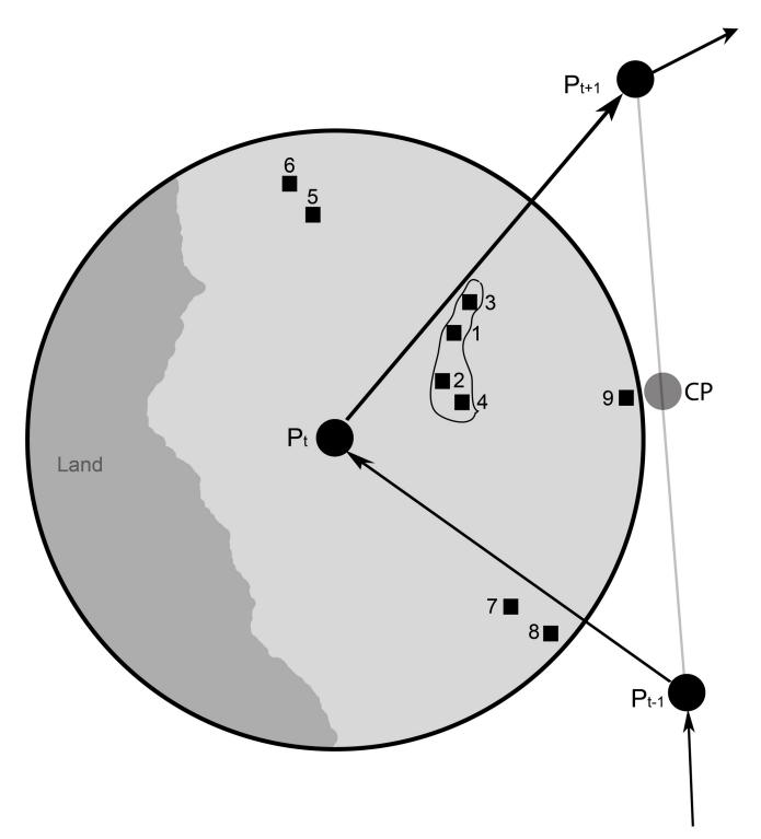
Fig 3. Search schematic of the genetic algorithm (GA). A circle of radius *R* is centered at the current position *P*<sub>t</sub>. The search area was constrained by land or shallow bathymetry. The numbers correspond to the nine scenarios outlined in the text.
