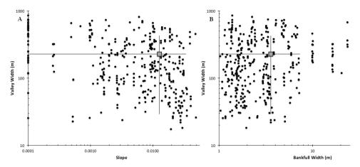
Fig 2. Geomorphic characteristics of stream segments in the Snohomish River Basin occupied by beaver. (A) Valley widths versus slope, (B) valley width v. bankfull width. Crosshair lines represent the standard deviations, and square symbols are the means. Note that the scale is logarithmic. The data show that dam-building beaver generally prefer streams with percent slope < 0.04, bankfull width < 8 m, and valley width > 30 m.
