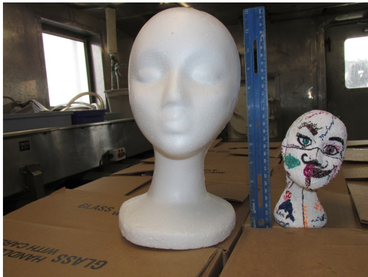
Figure 7. Styrofoam manikin heads, before and after 25 submersions down to as deep as 500 meters. This was a project undertaken by Prout High School oceanography students to demonstrate the effect that water pressure has on the gas bubbles within Styrofoam.
