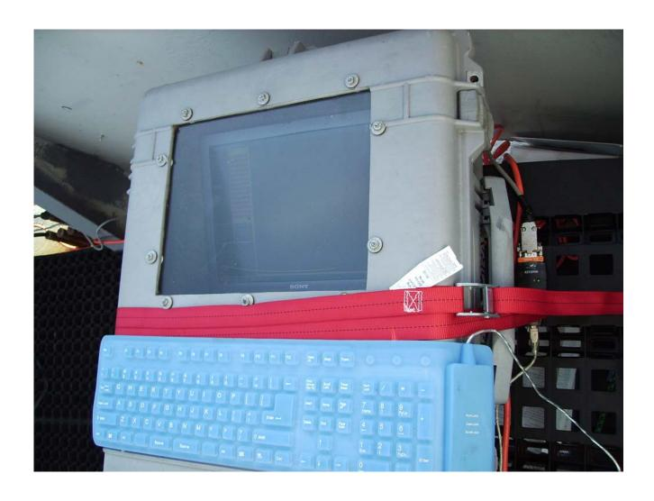
Figure 3. Waterproof data logging station for seabird and marine mammal observations on DELAWARE II flying bridge.
