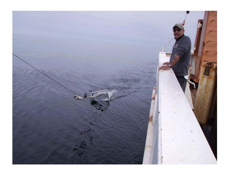
Figure 4. One half by one meter neuston frame equipped with 505 micron mesh net being deployed from the aft A-frame of the R/V DELAWARE II.
