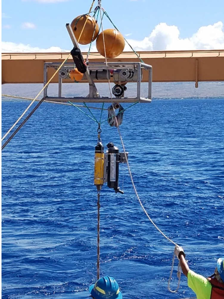
Figure 6.7 The MOUSS, Moana-360 (inside frame) and Ossolinski Actuator (attached to acoustic release) immediately before deployment from the NOAA Ship Oscar Elton Sette .
