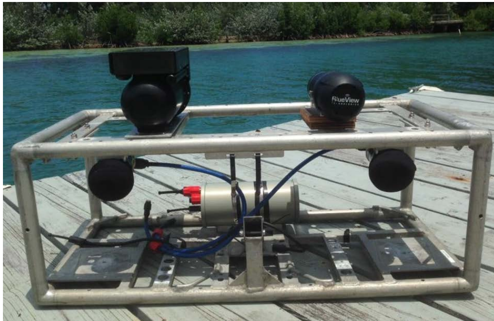
Figure 6.4 Configuration of the MOUSS-DIDSON inter-comparison study with the MOUSS mounted inside the frame, DIDSON mounted on top left, and BlueView (data not used) mounted on the top right of the frame.
