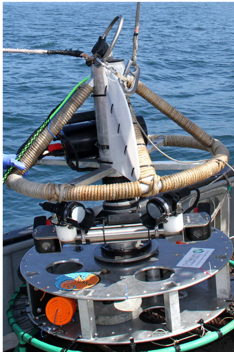
Fig 2. Stereo-video lander used to survey fishes in central California, U.S.A.
