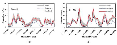
**Figure 4.** Calibration of observed and simulated streamflow (m<sup>3</sup>/s) during period (January 2010–December 2012): (a) Rio Guanajibo watershed, and (b) Rio Grande de Añasco watershed, Puerto Rico, USA.
