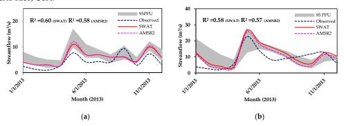
**Figure 6.** Validation of SWAT and AMSR2 streamflow (m<sup>3</sup>/s) with observed streamflow (m<sup>3</sup>/s) during period (January 2013–December 2013): (a) Rio Guanajibo watershed and, (b) Rio Grande de Añasco watershed, Puerto Rico, USA.
