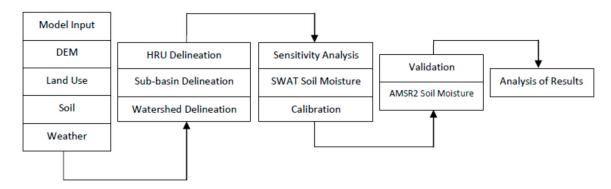
Figure 3. Flow chart of methodology for streamflow measurement using SWAT in Puerto Rico, USA.
