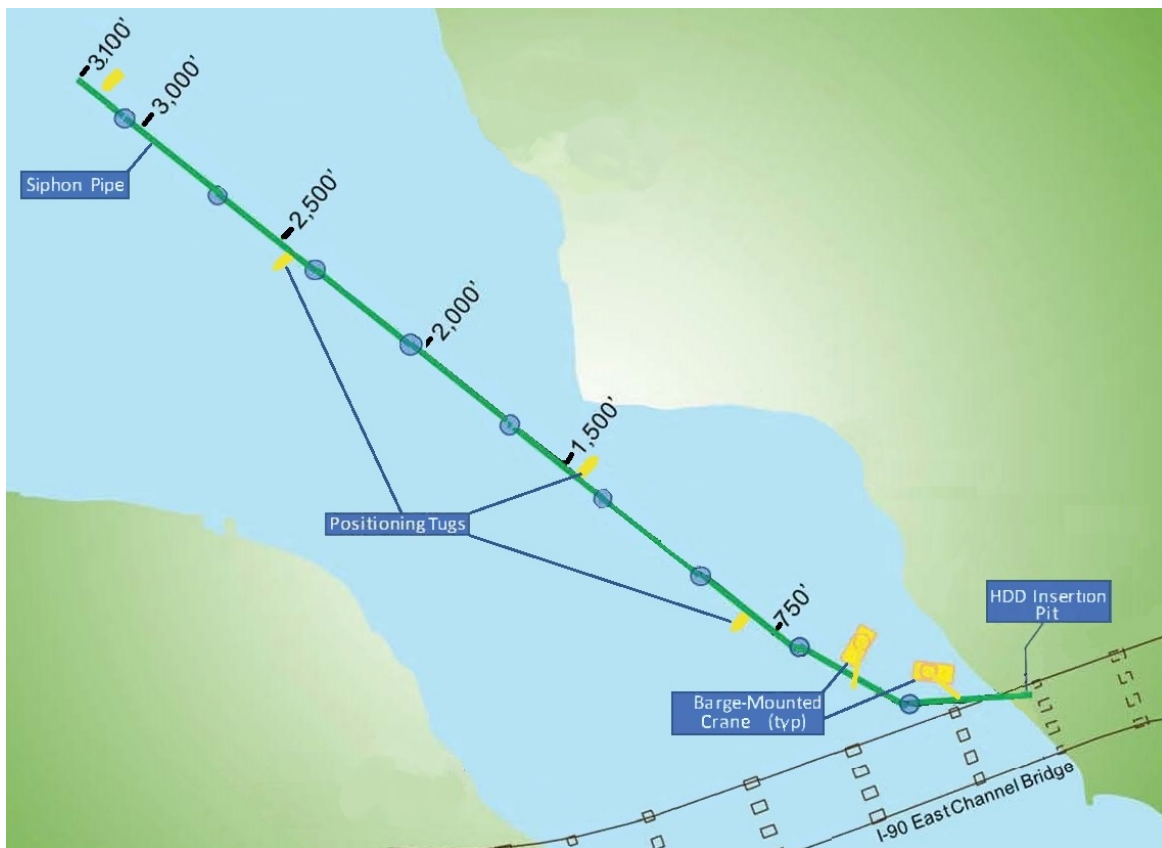
Figure 3. Approximate location the Enatai Siphon HDPE pipe floating on Lake Washington prior to it being pulled through the HDD borehole to the Swayolocken Pump Station (Adapted from Confluence 2019 Figure 14, per King County 2020b).
