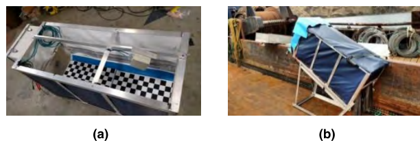
FIGURE 1. Chute with a static camera. (a) Interior view with checkboard for calibration. (b) Installation with cover on board.
