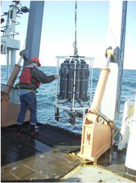
Figure 9. CTD 911 and rosette unit being deployed from aft A-frame of Delaware II.
