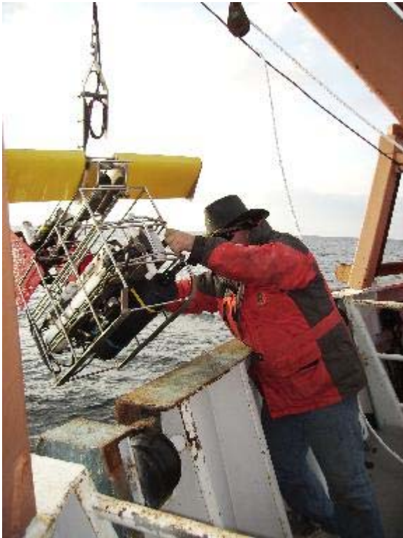
Figure 7. Crewmember Richard Logan launches Acrobat unit off the stern of Delaware II.
