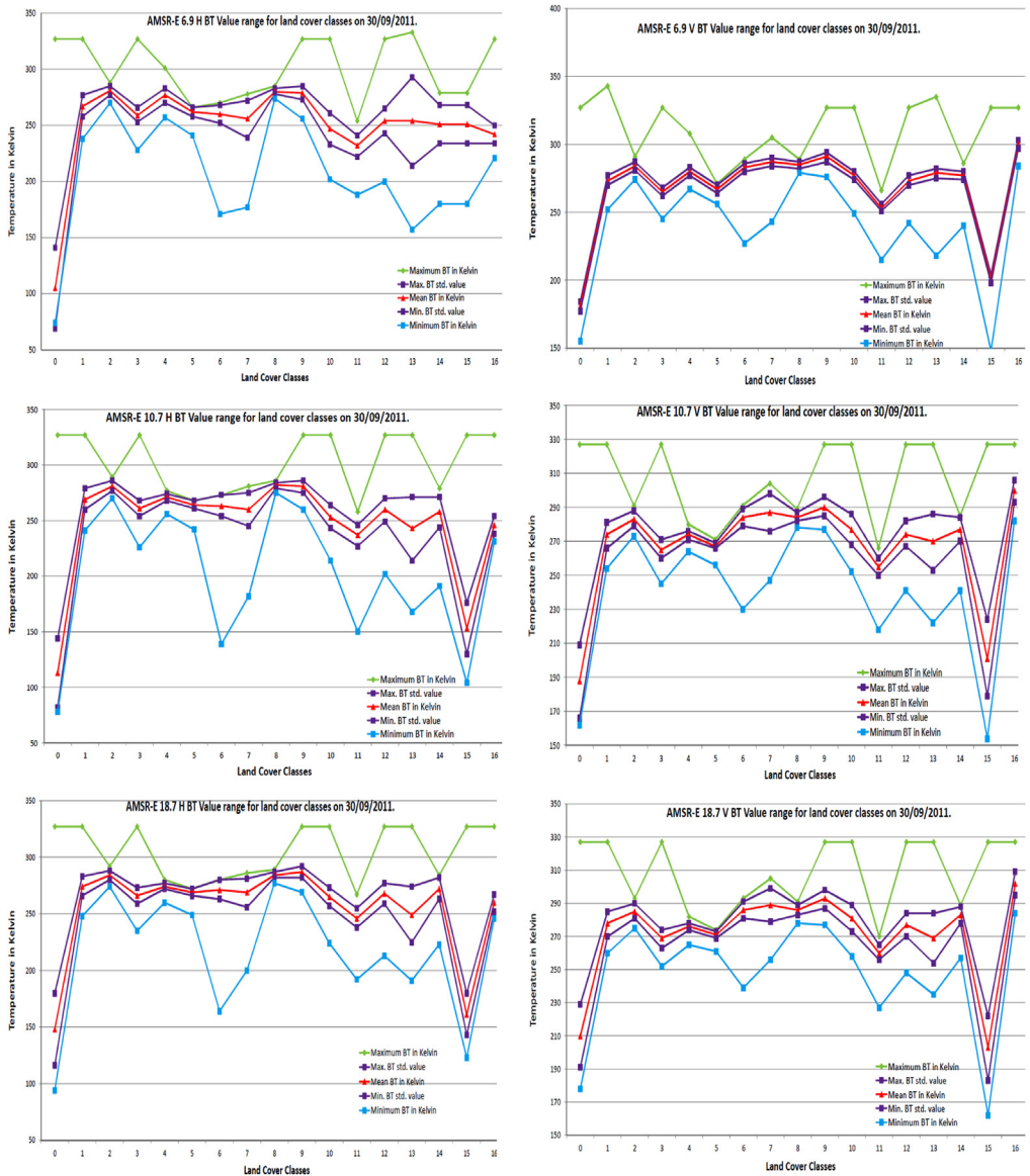
Fig. 3. Seventeen land cover classes maximum, minimum, mean and standard deviation temperature in kelvin for 6.9, 10.7, 18.7, 23.8, 36.5 and 89.0 GHz AMSR-E frequency.
