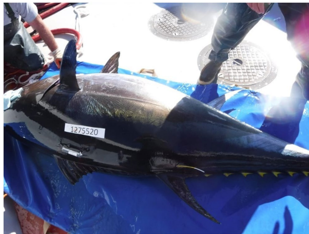
Figure 1. External acoustic tag attachment for an Atlantic bluefin tuna with two titanium darts in the dorsal musculature.
