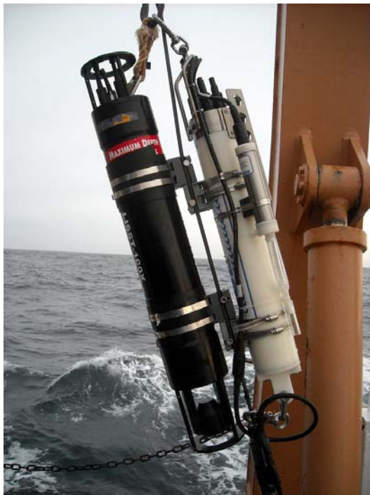
Figure 3. LISST (black cylinder) mounted on lower part of rosette frame.
