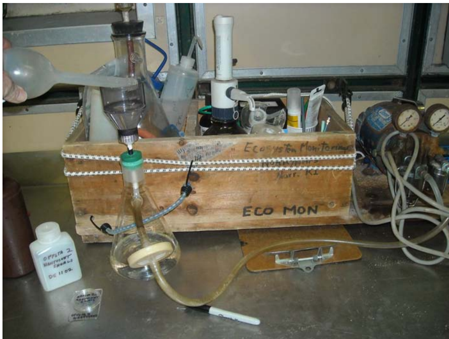
Figure 7. Filtering apparatus for nitrogen isotope and chlorophyll extraction.
