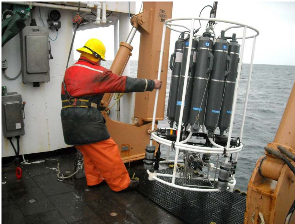
Figure 3. LISST (black cylinder) mounted on lower part of rosette frame.
