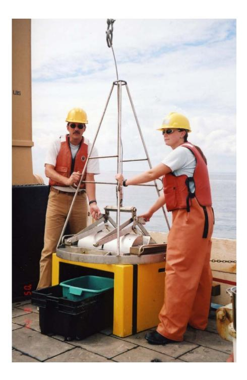
Figure 2. EPA scientists Don Cobb and Nora Sturgeon prepare to deploy a double Van Veen grab from the ALBATROSS IV.
