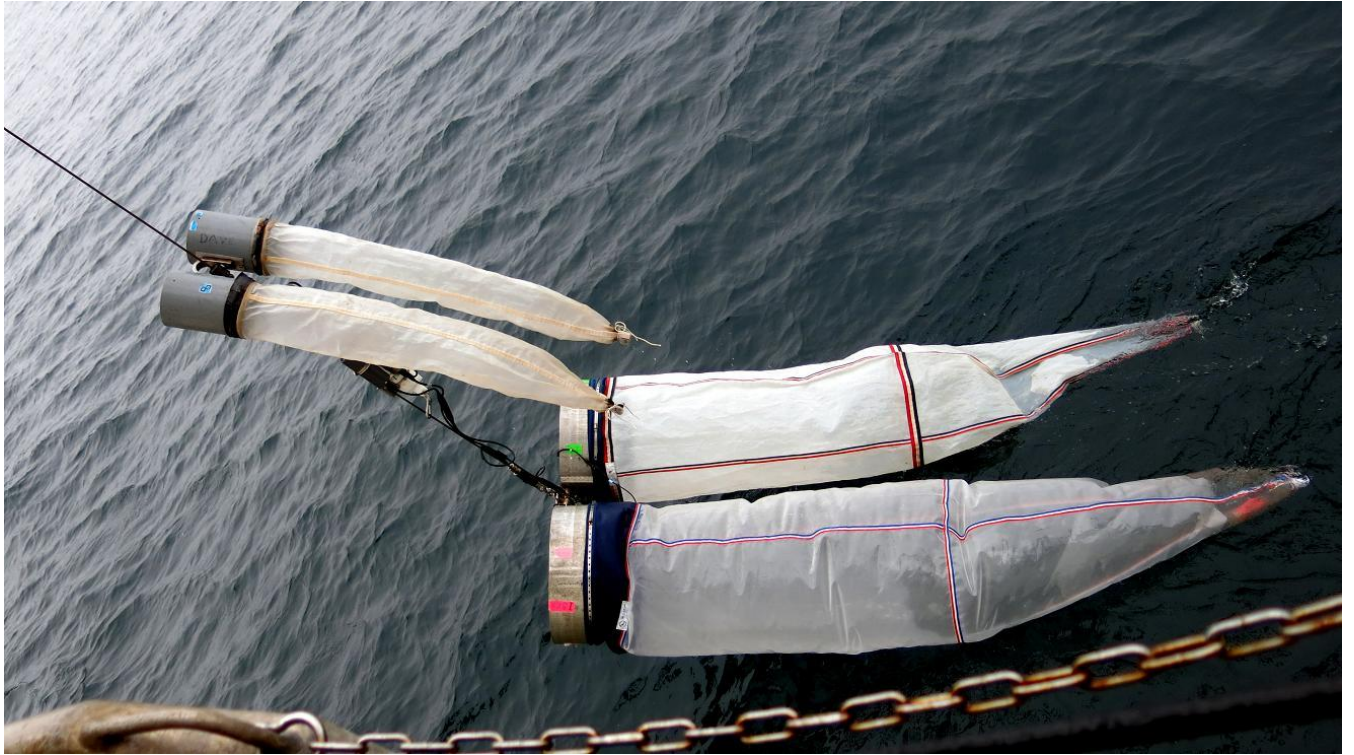
Figure 2. Bongo net array, showing 61 and 20 cm bongo nets being deployed from the HENRY BIGELOW Side Sampling Station. (DJ Kast photo).
