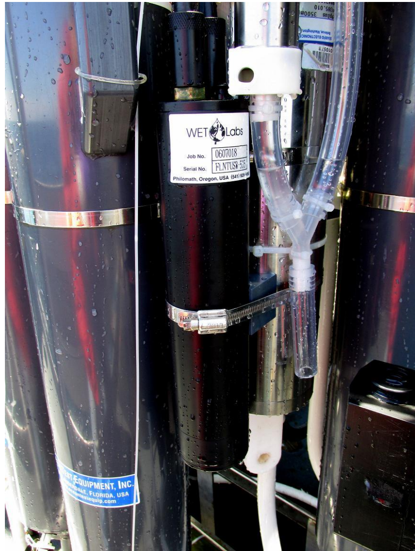
Figure 3. Wetlabs Fluorometer mounted next to a Seabird 19 Profiler CTD on a Niskin Bottle Rosette.
