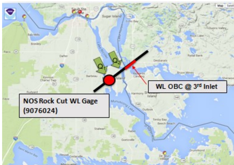
Figure 4. Map depicting the location where open boundary conditions were prescribed to take into account uncertainties in estimating inflow/outflow.
