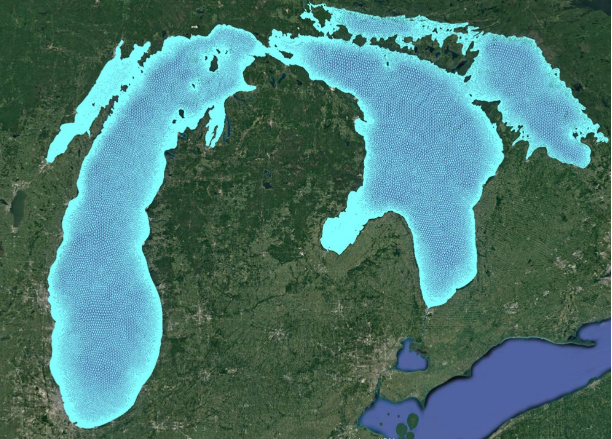
Figure 2. Map depicting the FVCOM grid domain for LMHOFS. The horizontal resolution ranges from 100 m (328 ft) near the shore to 2.5 km (1.6 mi) offshore with 21 vertical levels.
