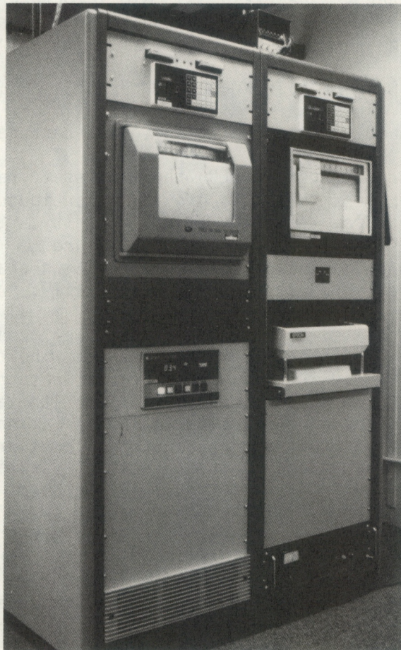
Figure 7.-- The completed installation of the M03 and ASR CAMS in Barrow. The M03 CAMS is in the left-hand rack above the wind recorder and dew point hygrometer.
