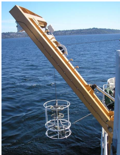
Figure 19. Photos of starboard side CTD deck showing J-Frame (left) and CTD Winch (right).
