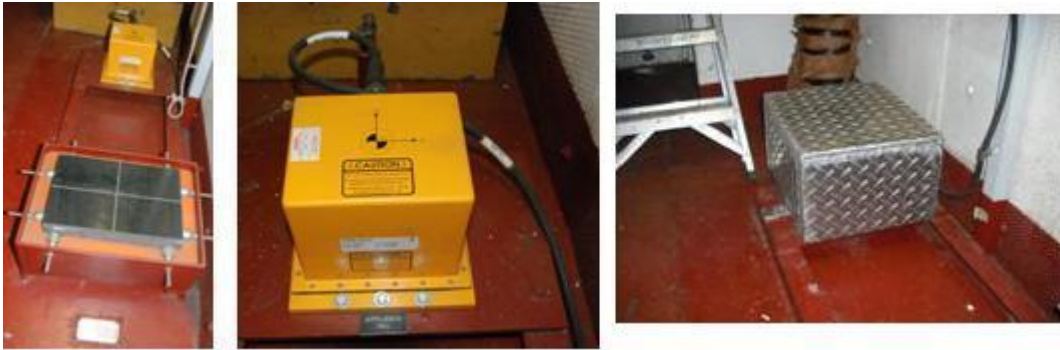
Figure 6. Photos: From left: IMU and granite block, IMU, IMU under protective housing.
