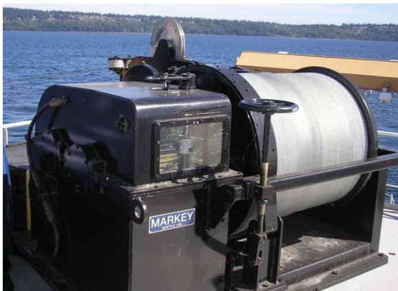
Figure 19. Photos of starboard side CTD deck showing J-Frame (left) and CTD Winch (right).
