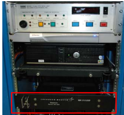
Figure 8. Photos: XBT launch from the aft deck (left). Deck unit for XBT in red (right)
