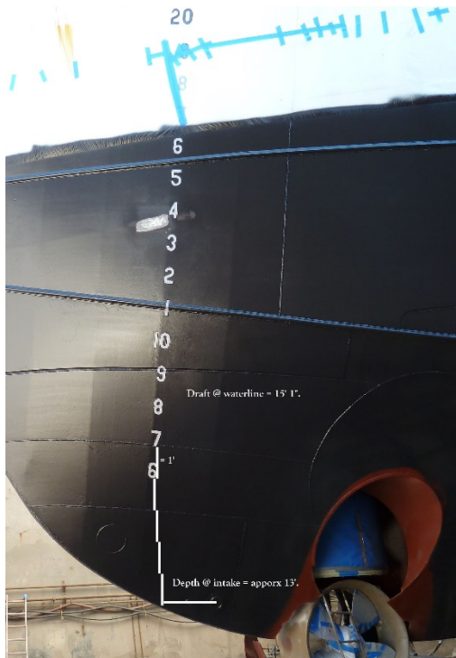
Figure 12. Photo showing depth of TSG intake location on the hull, approximately 13 feet below the water line.
