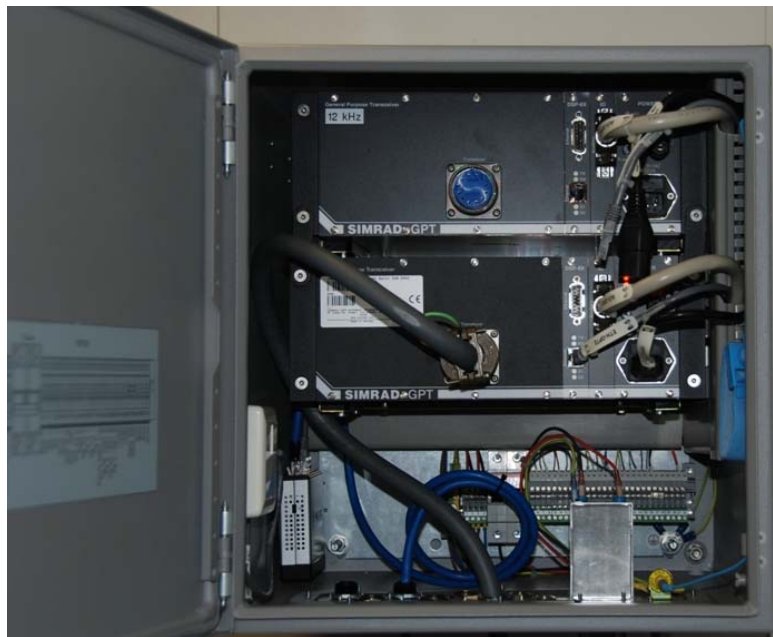
Figure 2. EK 60 (bottom) / EA 600 (top) (disconnected) GPTs.
