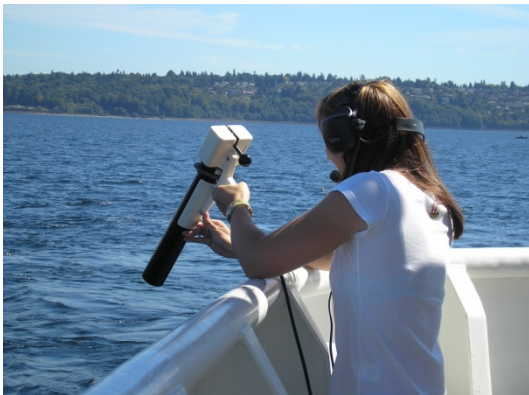
Figure 8. Photos: XBT launch from the aft deck (left). Deck unit for XBT in red (right)
