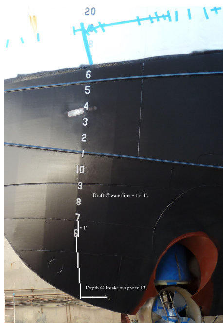
Figure 11. Photo showing depth of TSG intake location on the hull.
