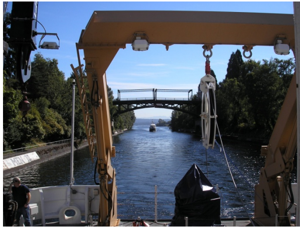
Figure 2. Photo looking aft showing A-Frame.
