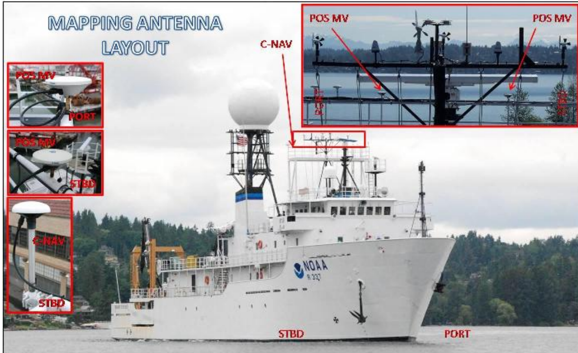
Figure 8. Photos: POS/MV antennas mounted on the Flying Bridge (below). Also shown is the CNAV antenna.
