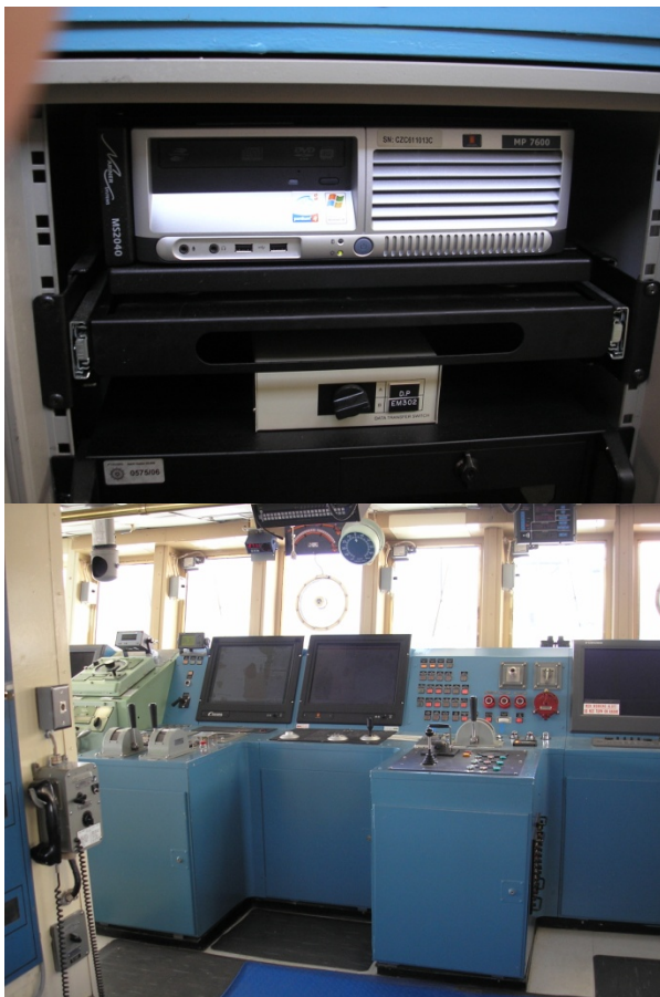
Figure 15. Bridge DP system installed on Okeanos Explorer showing different controls and the USB drive for inputting electronic files for the way point table.
