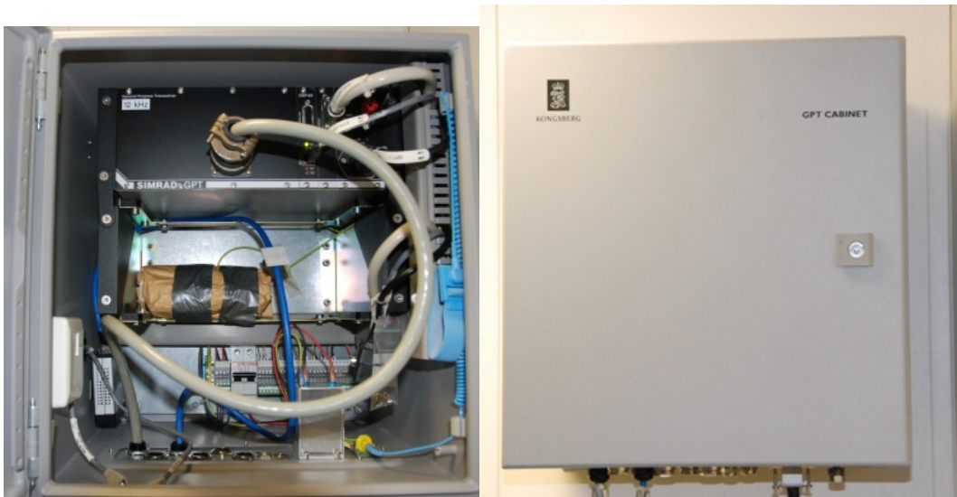
Figure 6. Photos showing EA600 TRU interior (left) and EA600 TRU outer casing (right).
