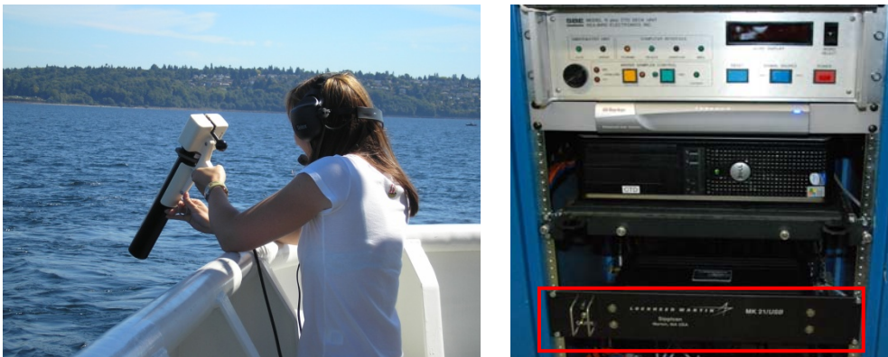
Figure 10. XBT launch from the aft deck (left). Deck unit for XBT (right)
