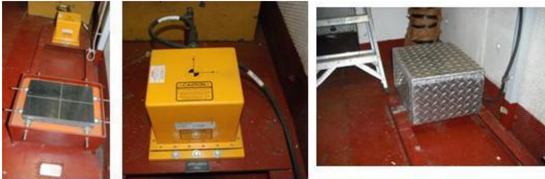
Figure 8. Clockwise from top left: IMU and granite block, IMU, IMU under protective housing.
