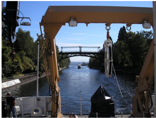
Figure 2: View of A-Frame looking aft. The A-Frame is presently configured to handle the ROV.
