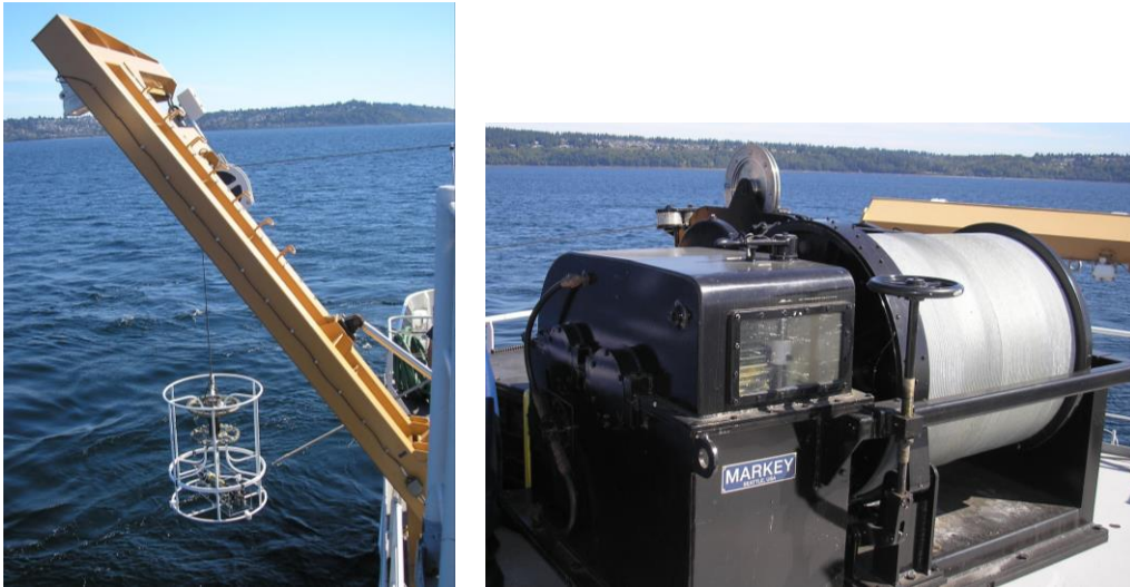
Figure 1: J frame located on starboard side is designed for CTD casts (left). CTD Winch (right).
