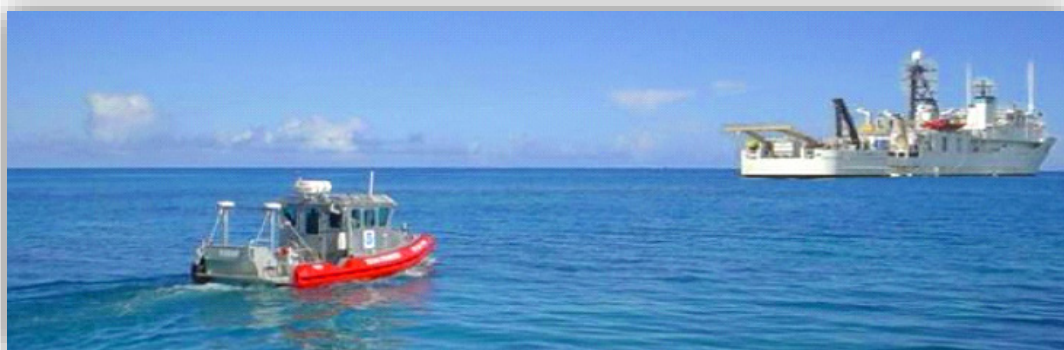
Figure 8. The survey launch R/V AHI and NOAA Ship Hi'ialakai were outfitted with multibeam echosounders that facilitated multibeam surveys across the Pacific Islands Region.
