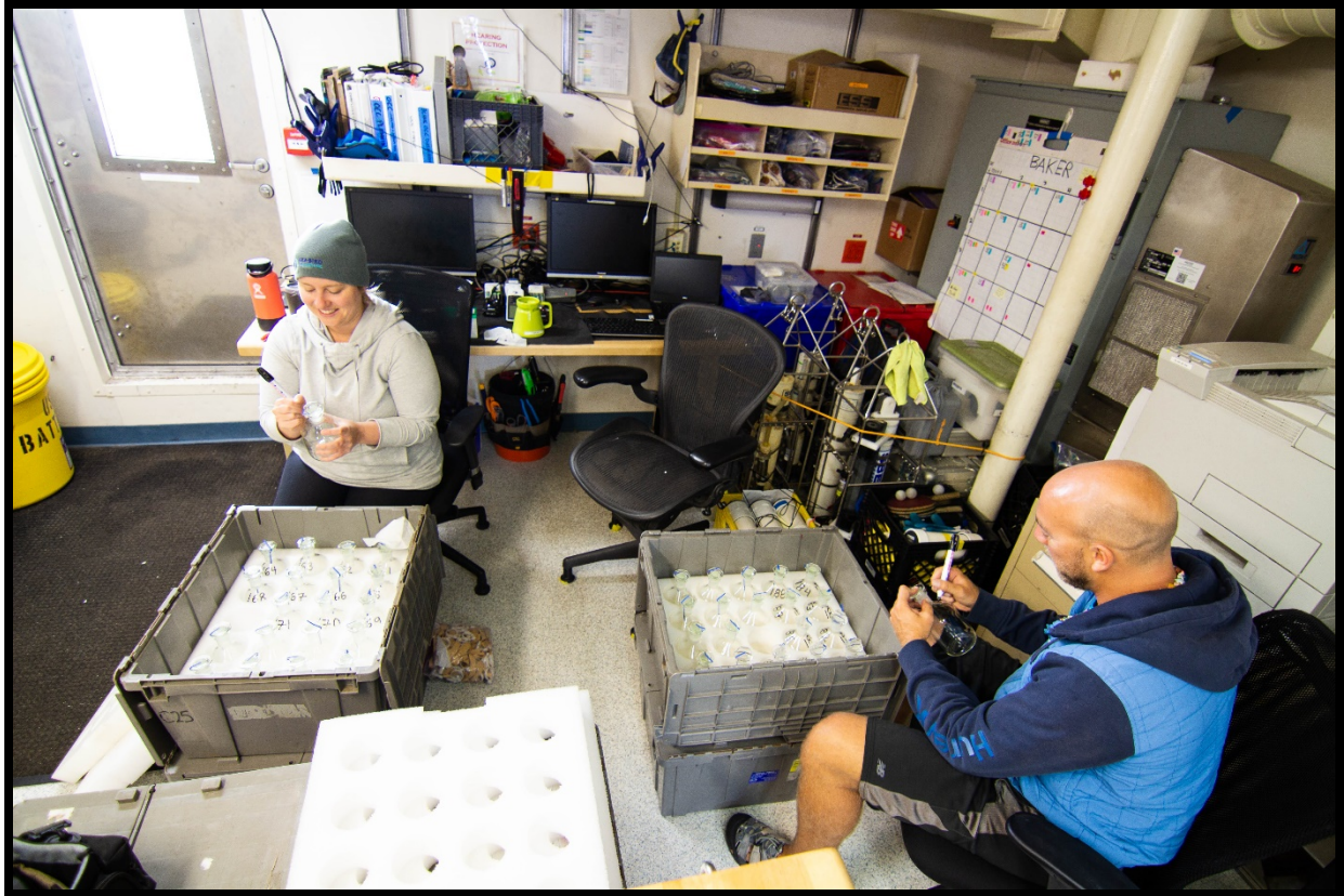
NOAA scientists Hannah Barkley and Ariel Halperin prepare equipment for use by the ocean and climate change team at Howland Island. These bottles will be filled with water samples to measure dissolved inorganic carbon composition in the ocean.
