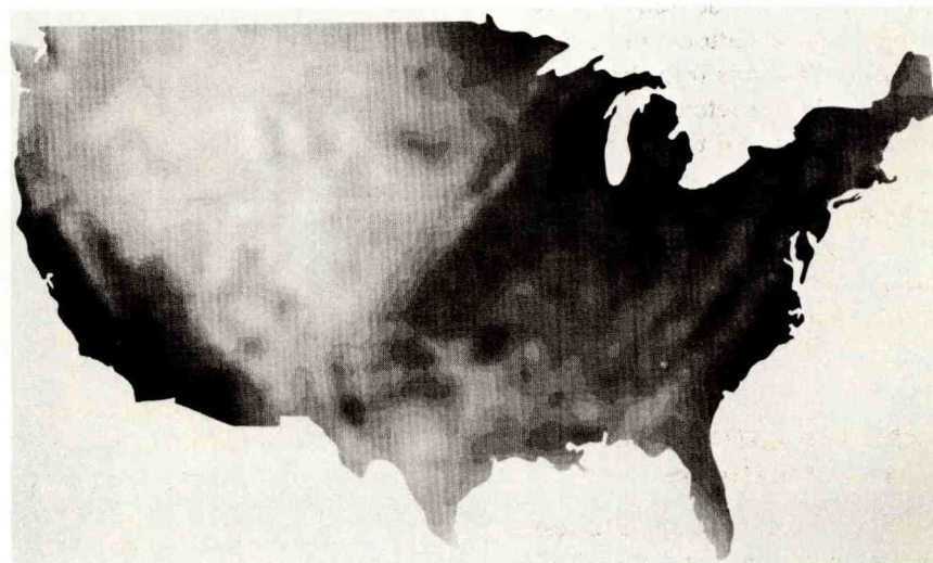
Undulations of the geocentric geoid represented by gray shades, range from -37 m (black) to -10 m (white).
