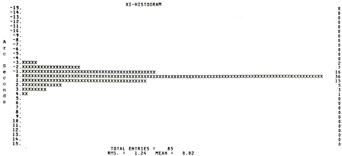
Figure 24. —Distribution of Residual Differences in Meridian in area \phi=39^\circ - 44^\circ , \lambda=116^\circ - 125^\circ
