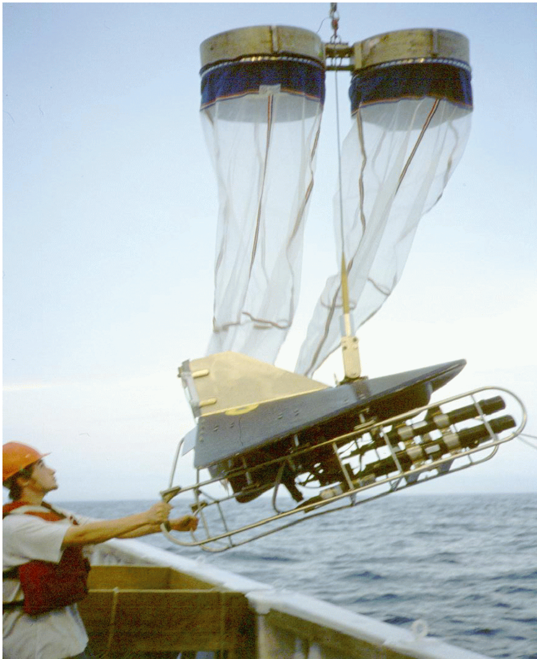
Figure 4. Bongo and VPR Sled being deployed during AL0207 Part 1: Bongo-VPR Comparison Leg, 11 - 15 June 2002.
