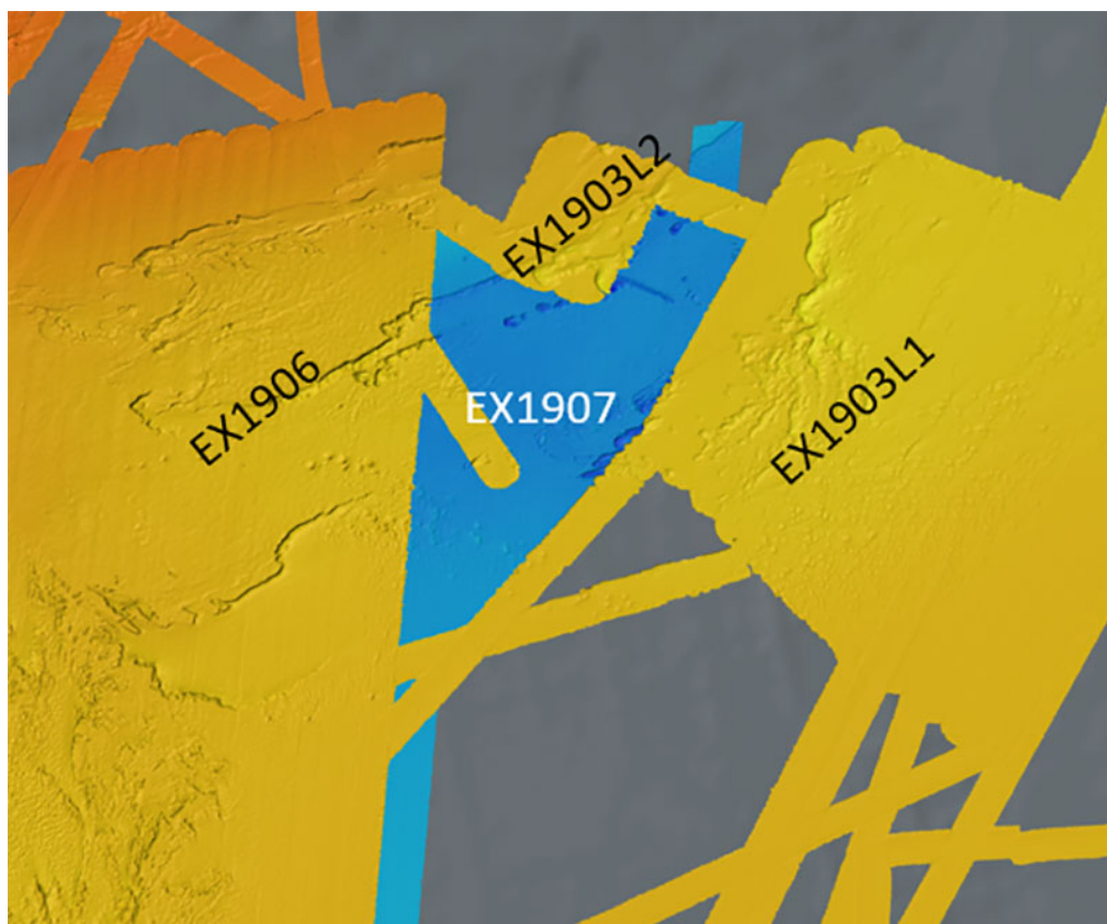
Figure 3. Example of mapping optimization during overnight operations and weather days. Mapping operations were able to fill in an unmapped area and merge it with mapping data from three previous Okeanos Explorer cruises in the region: EX1903L1, EX1903L2, and EX1906.
