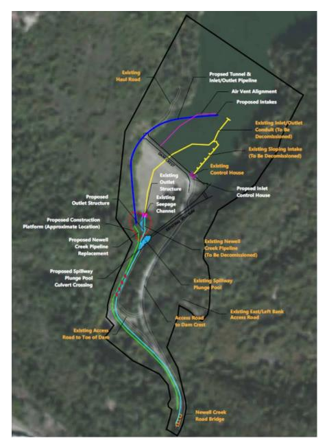
Figure 1. Map of existing and proposed project facilities/components for the Newell Creek Dam Inlet/Outlet Replacement Project. The red dots downstream of the plunge pool are the approximate locations of the existing failed log weirs proposed for replacement as part of Mitigation Project 3.
