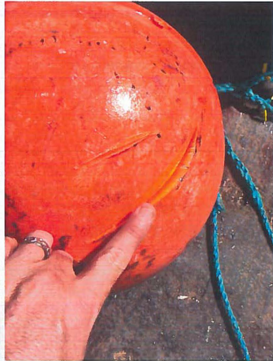
Figure 4 DCIP sub-surface float showing evidence of propeller strike.
