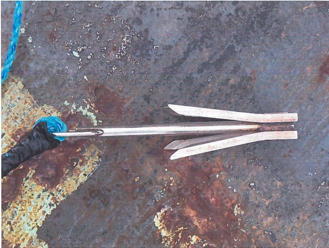
Figure 2 An image of the "line pinching" grappling hooked used to attempt recovery of the MOUSS.
