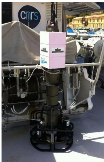
Figure 2-3. This nke Instrumentation PROVOR float hosts a pH optode sensor developed by TU Graz and Pyro Science (photo courtesy of Arnaud David).
