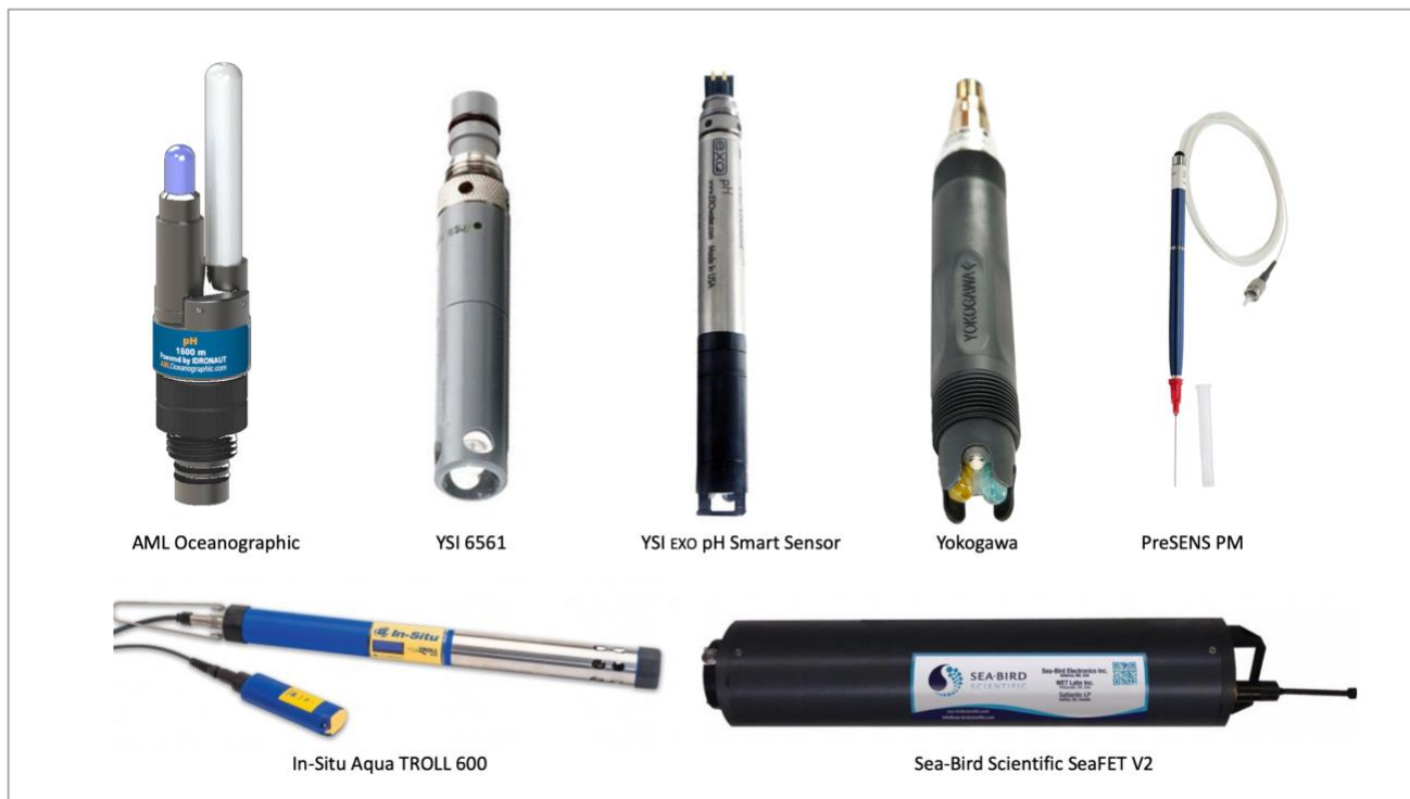
Figure 2-4. Some commonly used pH sensors (photos courtesy of vendors).
