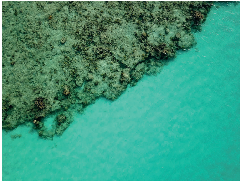
Figure 3.4. Example of benthic features with high bottom texture (upper-left of the photo) and low bottom texture (bottom-right of the photo) in St. Croix. Higher amounts of bottom texture are critical for SfM to match and align images, and map seafloor depths. SfM will create inaccurate depths over geographic locations that are featureless and have low bottom texture.
