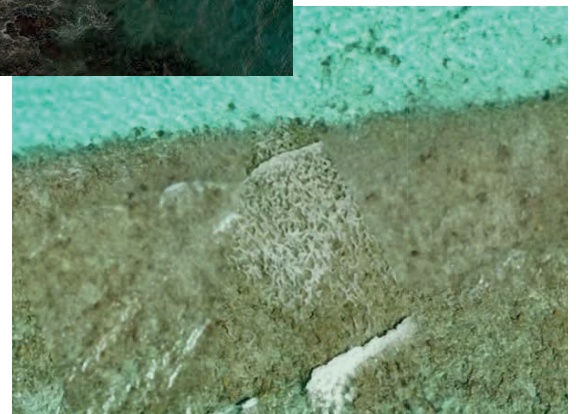
Figure 3.6. Example of whitewater in Santa Cruz Island (top) and St. Croix (bottom). Breaking waves and whitewater (as seen in these images) obscure the seafloor, reducing the ability of SfM to match and align images and accurately map depths.
