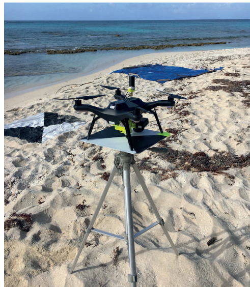
Figure 4.5. If a GCP is used as the takeoff/landing site, it can be surveyed using the sUAS GNSS and utilized as a GCP without the need for additional survey hardware. Here, a 3DR Solo with PPK demonstrates this technique on St. Croix.
