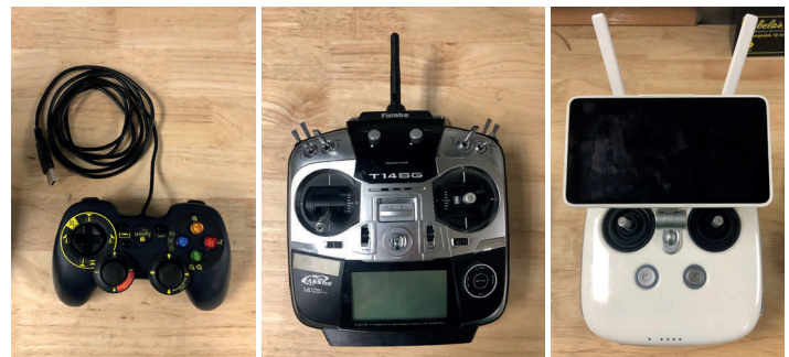
Figure 2.3. Three common style of sUAS controllers are video-game style controllers (left), traditional RC style controllers (middle), and custom controllers from the sUAS manufacturer(right).
