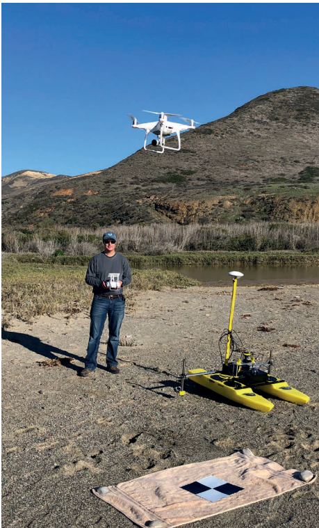
(Right) Chris Parrish (OSU) pilots the DJI Phantom 4 Pro RTK sUAS on Santa Cruz Island, CA. The Seafloor Systems HyDrone ASV is seen in the foreground. (Middle) Project team plans and adjusts mission based on real time weather conditions north of St. Croix. (Right) Tim Battista (NOAA NCCOS) deploys GCP target in shallow water offshore of Buck Island, St. Croix. Photo Credits: Oregon State University and NOAA NCCOS.
