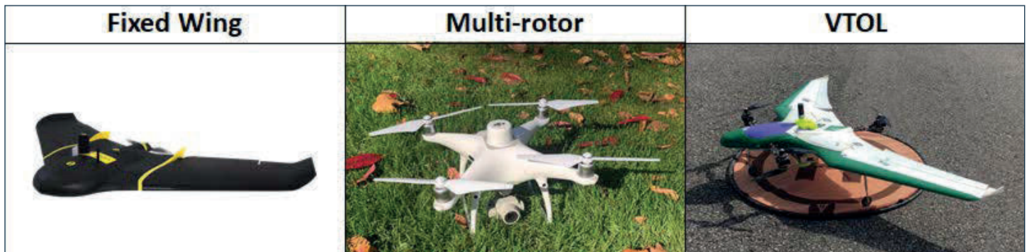
Figure 2.1. The three main types of airframes are fixed-wing (left), multirotor (middle), and vertical takeoff and landing (VTOL; right). Credit: senseFly, Oregon State University, and C.W. Wright
