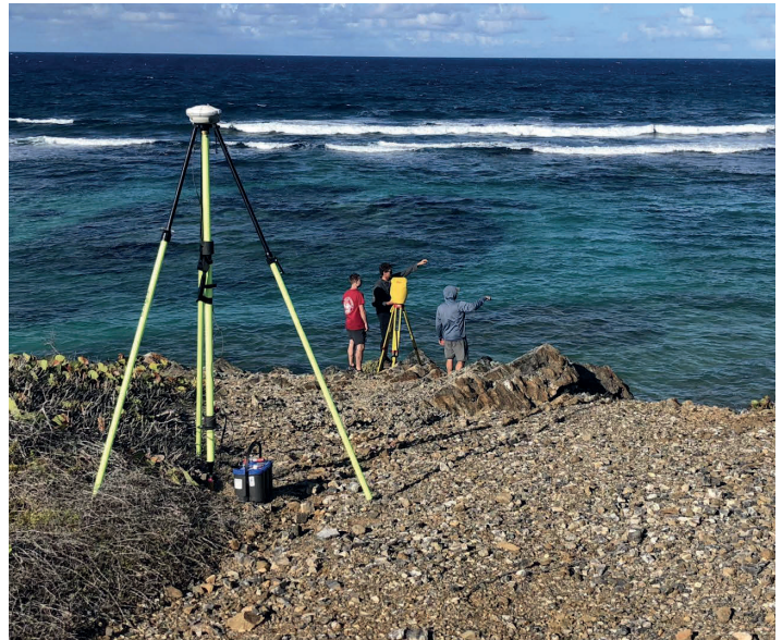
Figure 7.10. The Whale Point, USVI field site experienced large errors in some of the processed datasets, which could have been due to the wave action in the area of interest. Here members of the project team (L-R: Matt Sharr, Chase Simpson, and Bryan Costa) organize a survey plan for acquiring a ground truth dataset. Credit: Oregon State University.
