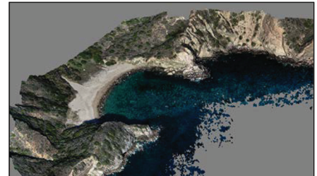
Figure 3. A 3D model created using sUAS imagery and SfM software for Coches Preitos Anchorage. This model will be processed further into absolute elevations and depths.
