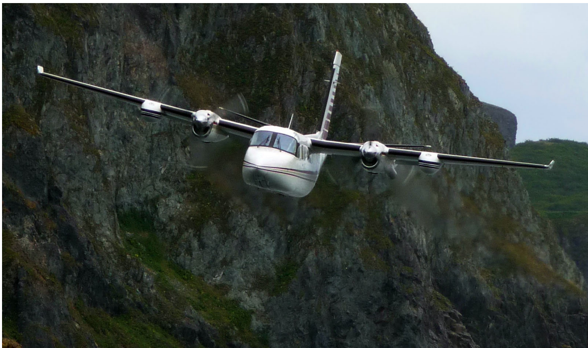
Figure 2. -- Twin engine, high wing Aero Commander 690 survey platform used during Cook Inlet beluga aerial surveys, June 2018 (photo courtesy of Clearwater Air, Inc.).
