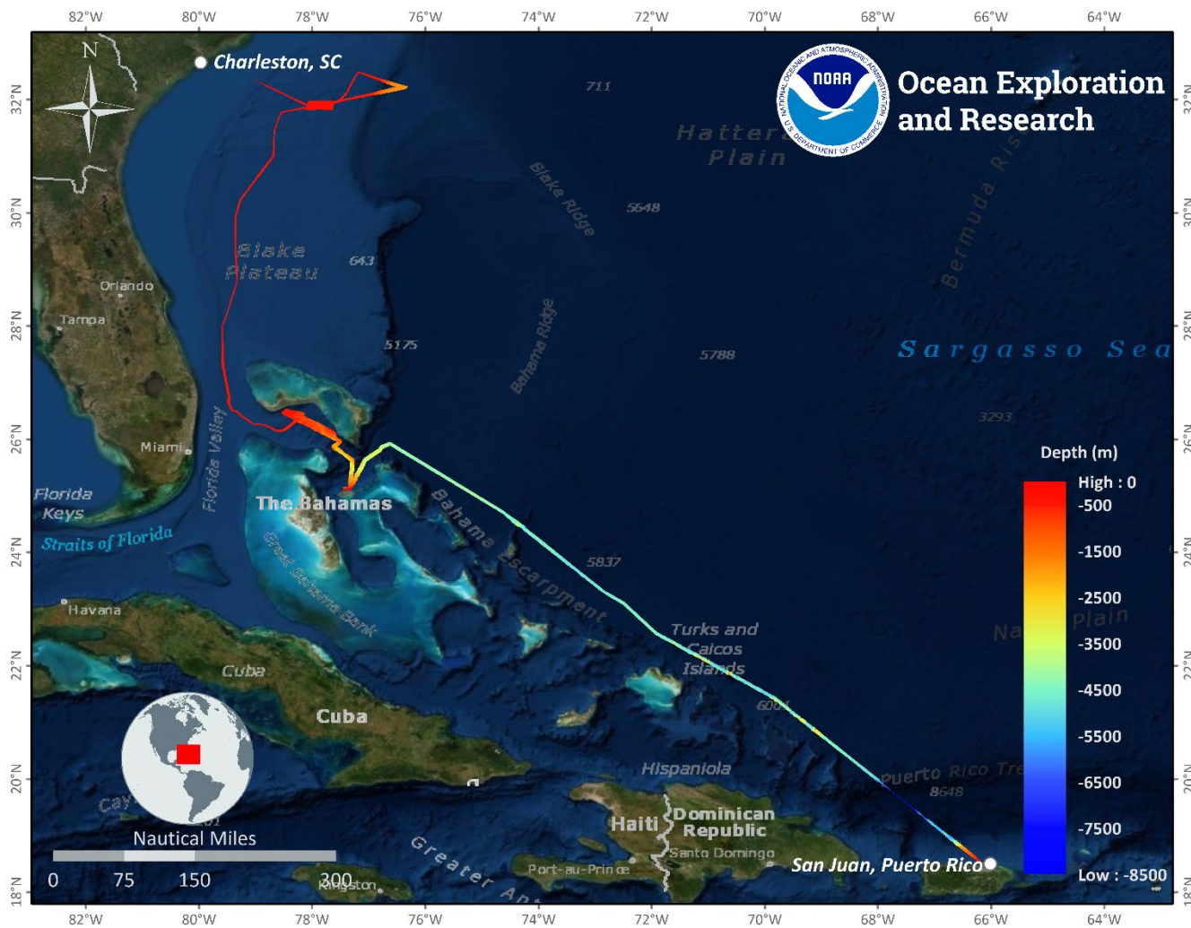
Figure 1. Overview map showing bathymetry mapping coverage completed during the 2018 Mapping Deepwater Areas in the Caribbean and South Atlantic Bight (EX-18-12). Map created by NOAA Office of Ocean Exploration and Research (NOAA-OER), generated in ArcMap.
