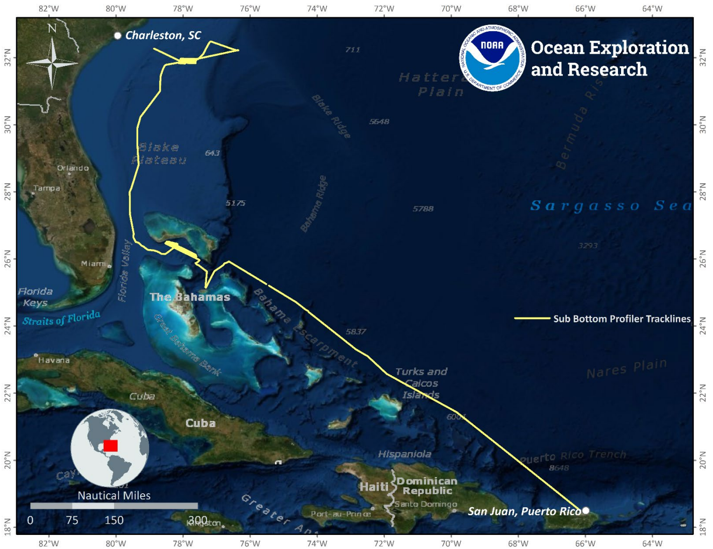
Figure 3. Overview showing tracklines of Knudsen sub-bottom profiler data (in yellow) collected during the first leg of the 2018 Mapping Deepwater Areas in the Caribbean and South Atlantic Bight (EX-18-12). Map created by NOAA Office of Ocean Exploration and Research (NOAA-OER), generated in ArcMap.
