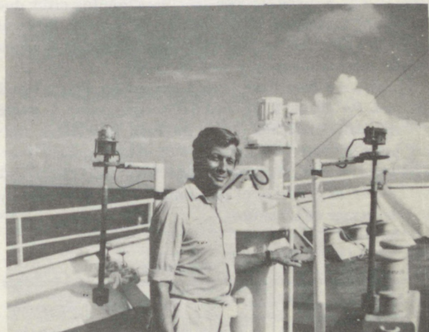
FIG. 1. Installation on the bow of the E. Krenkel of an Eppley (Model 2) pyranometer and Yanishevsky (Model M-80) pyranometer on identical gimballed mounts. Mr. E. I. Druzhinin of the Main Geophysical Observatory, Leningrad, U.S.S.R., who was responsible for the installation is shown in the photo.
