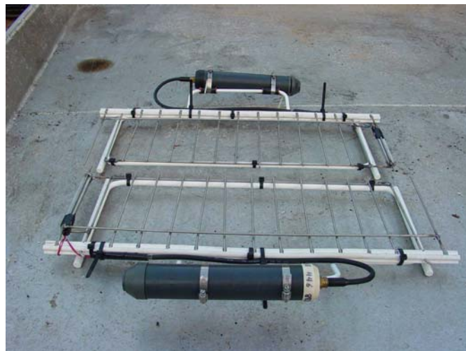
Figure 7. Two modular trigger assemblies with trigger timers mounted.
