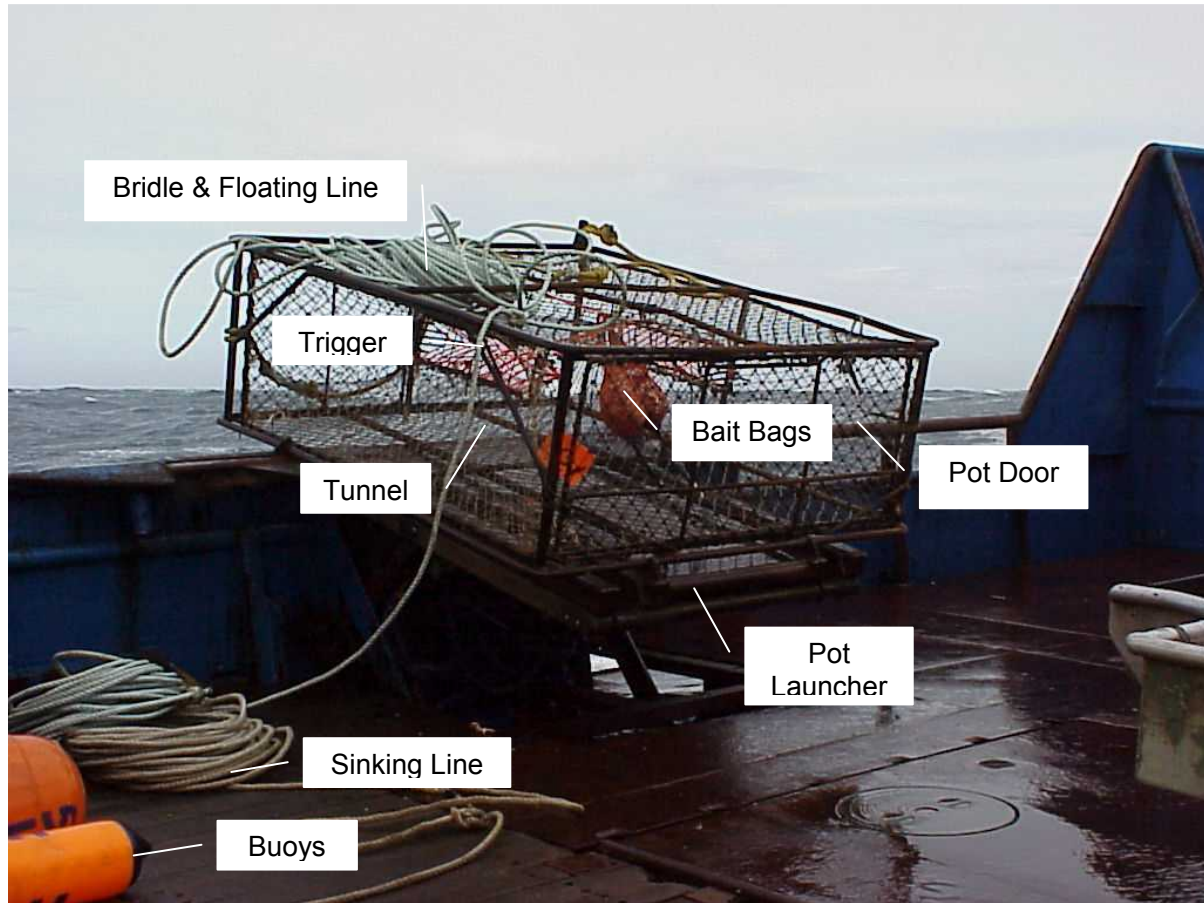
Figure 6. Commercial cod fishing pot in pot launcher. Bait is suspended in the center of the pot. Fish enter the pot by swimming up the indented tunnels and pushing through one-way triggers (orange “fingers” in photo).
