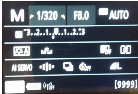
Figure 1. Canon SL2 LCD monitor displaying correct settings for SfM image collection.
