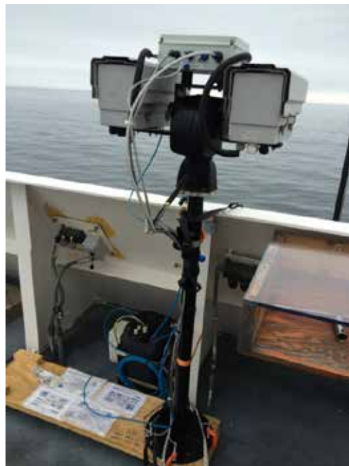
Figure D2. Photograph of infrared camera setup on the flying bridge for HB15-03 Leg 1.
